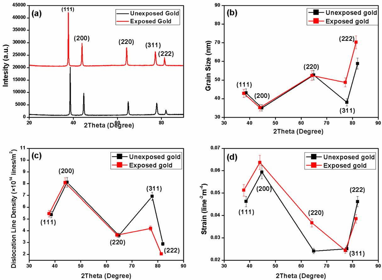
Figure 2: A plot of Bragg's angle 2(theta) vs (a) diffracted x-ray intensity (b) dislocation line density (c) grain size (d) strain, for un-irradiated and irradiated gold
