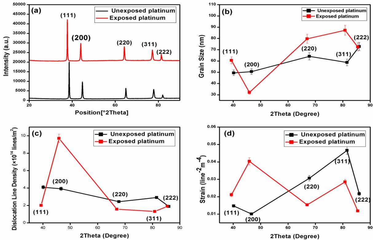
Figure 4: A plot of Bragg's angle 2(theta) vs (a) diffracted x-ray intensity (b) dislocation line density (c) grain size (d) strain, for un-irradiated and irradiated platinum
