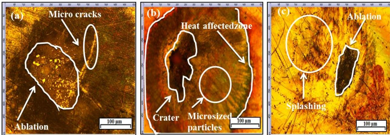
Figure 1: Optical micrograph (10x) of irradiated (a) gold (b) copper (c) platinum, for 200 laser shots
